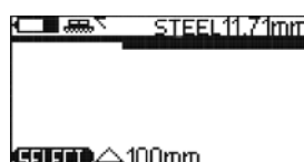
Figure 2.8 - Measurement mode with the B-Scan output
